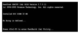
2. Press the Ctrl-F keys to display the FastBuild Utility Main Menu (below).
